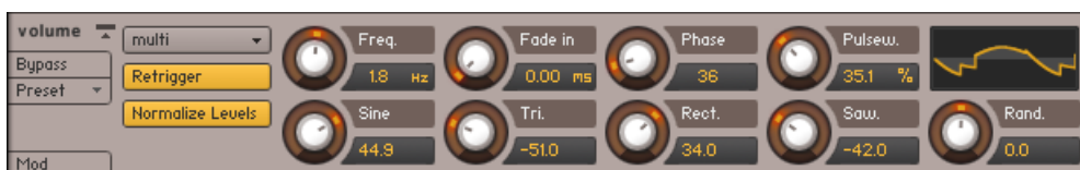
A Multi LFO, which lets you mix all other waveforms into a complex waveform.
